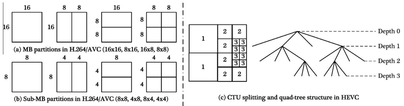
Fig. 1. Block partitions in H.264/AVC and CTU splitting, quad-tree structure in HEVC.
