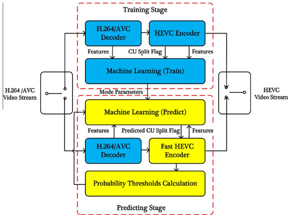
Fig. 5. Framework of the proposed H.264/AVC to HEVC transcoding.
