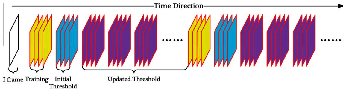
Fig. 9. Adaptive threshold updating mechanism.
