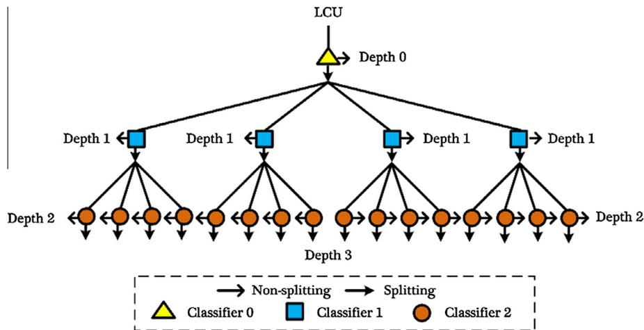
Fig. 4. CU splitting or non-splitting model in HEVC.
